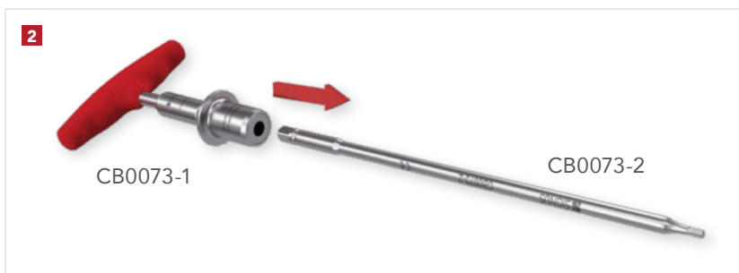
Connect the T-Handle with torque limiter 3 Nm with the set screwdriver.
