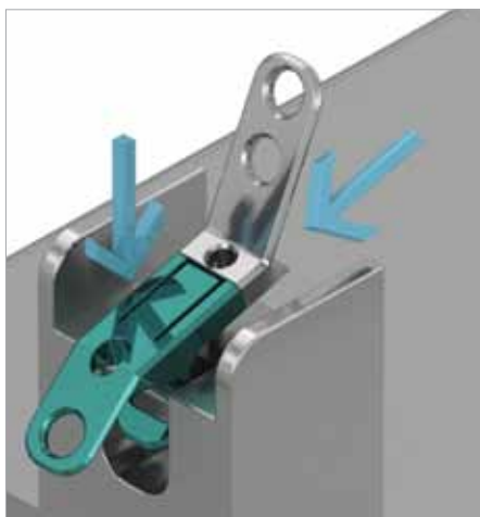
Push Down on Green Side, while Sliding Grey Side Closed
